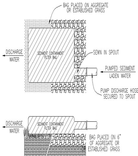
For larger amounts of water an operator may require a containment structure such as the one shown in the upper right. The intent of such a structure is to handle large amounts of pumped water and facilitate sediment removal. Structures must be sized appropriately for the pump or pumps total capacity. The lower right shows an alternative dewatering structure that can be constructed from materials most contractors have on hand. This structure is adequate for most situations.
