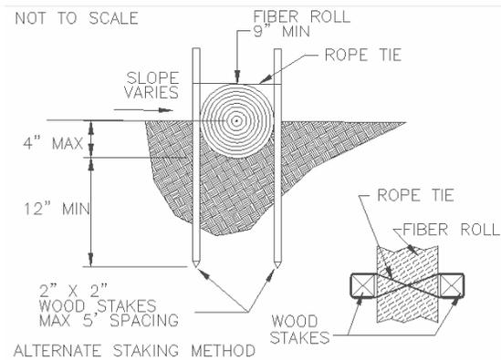
Fiber rolls consist of straw or wood fiber contained in netting to form a log shape. They are 9"-20" in diameter. They must be secured with stakes. Typical installation requires that rolls be entrenched. It is important not to crush fiber roll when it is installed.
